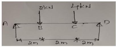
b. Draw the shearing force and bending moment diagrams for the beam in figure and identify salientfeatures.
