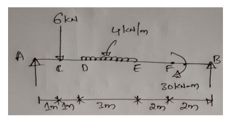
b. Draw the shearing force and bending moment diagrams for the beam in figure and identify salientfeatures.
