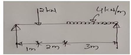
a. Draw the shearing force and bending moment diagrams for the beam in figure and identify salientfeatures.
